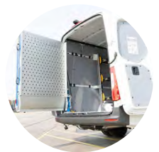
Standard left-hand swivel pivots the ramp, allowing easy cargo area access.
