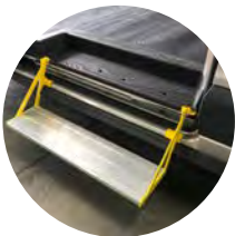
Aluminum step surface, with horizontal lines for traction assistance
