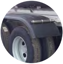
Tandem fenders are designed to span the length of two axles
