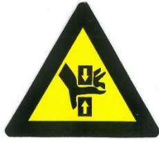
Risk of crushing
